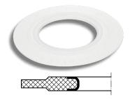
Optimized flat gasket made of multi-directionally stretched ePTFE with inner eyelet [TFM™ 1600]. The outer area is pre-compressed. Ideal for stress-sensitive flange systems such as plastic, glass or GRP flanges. Application parameters range from -268°C to 230°C [up to 315°C for brief peri-ods] and max. 40 bar.
