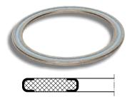
PTFE gasket made of modified, cold flow-reduced Dyneon<sup>TM</sup> TFM<sup>TM</sup> 1600 without fillers, with inner and outer eyelets. The double eyelet surrounds the TFM<sup>TM</sup> and prevents the material from settling or flowing in the tongue and groove area. The application limits range from  $-200^{\circ}$ C to  $200^{\circ}$ C and max. 40 bar.
