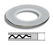
This envelope gasket with internal diffusion barrier combines the outstanding material properties of PTFE with the excellent leakage rate of the corrugated stainless steel ring. Leak-tightness is achieved even at a low surface pressure since the diffusion barrier is injected first. The benefit of this is the extremely low leakage rates at high operating parameters of -268°C to 250°C [up to 300°C for brief periods] and max. 80 bar.
