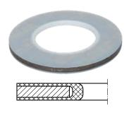
This envelope gasket combines the excellent material properties of PTFE with the adaptability of a non-metallic gasket. Particularly suitable for use in enamel flanges. Insert available in aramid fiber, graphite [SIGRAFLEX® EMAIL] or PTFE [UNIFLUOR®]. The demanding requirements of FDA and EC1935/2004 [EU10/2011] are reliably fulfilled, especially in combination with UNIFLUOR®.
